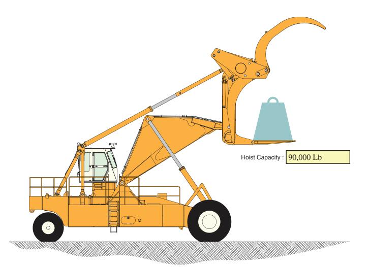
Verify that the machine can hoist the rated load. Secure back end before testing.
