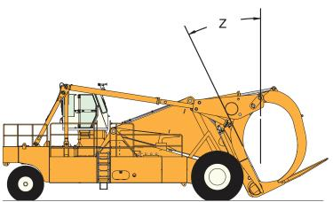
Carriage Angle from Vertical - Hoist Fully Extended, Tilt Fully Retracted (X): 42° 48° 81
