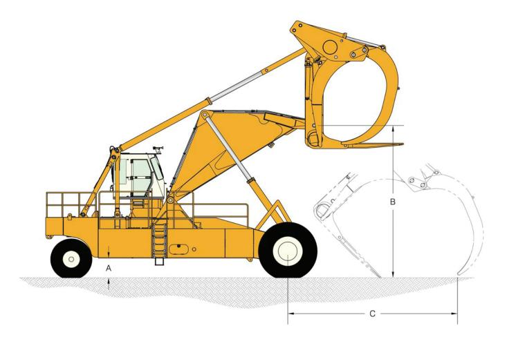
Ground Clearance, Chassis (measure from rear of chassis side tank) (A)
