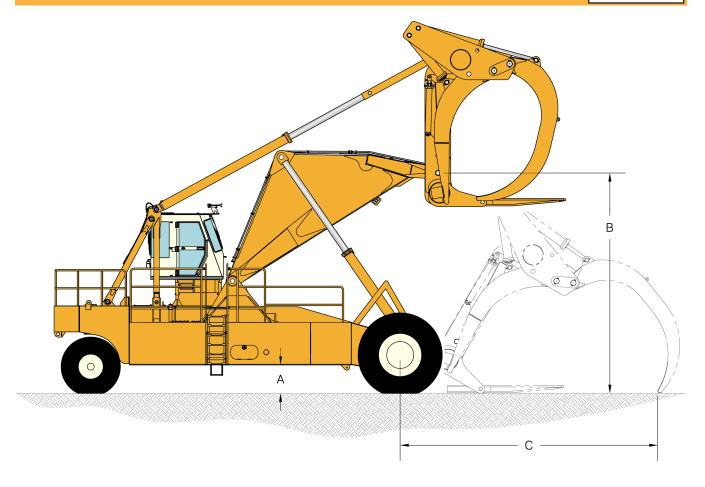
Ground Clearance, Chassis (A): Ground to Carriage Pivot Pin at Maximum Hoist (B):
