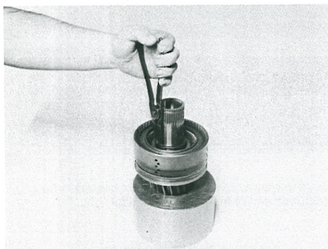
Figure 74 Remove low gear bearing locating ring.
