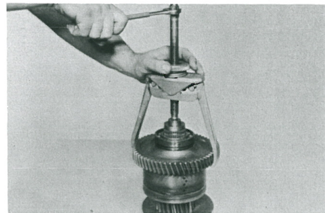
Figure 72 Remove low gear and hub, bearing spacer and low clutch front bearing.
