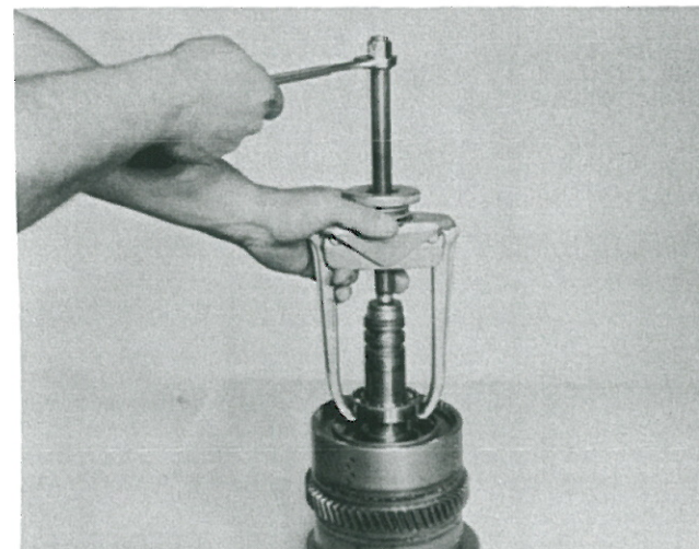
Figure 102 Remove inner bearing.
