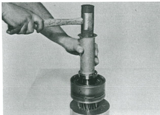
Figure 90 Install low speed gear inner bearing.
