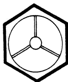
Grade 5 Identification 3 Radial Lines 120° Apart on Heads of Bolts.
