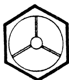
Grade 5 Identification 3 Radial Lines 120° Apart on Heads of Bolts.
