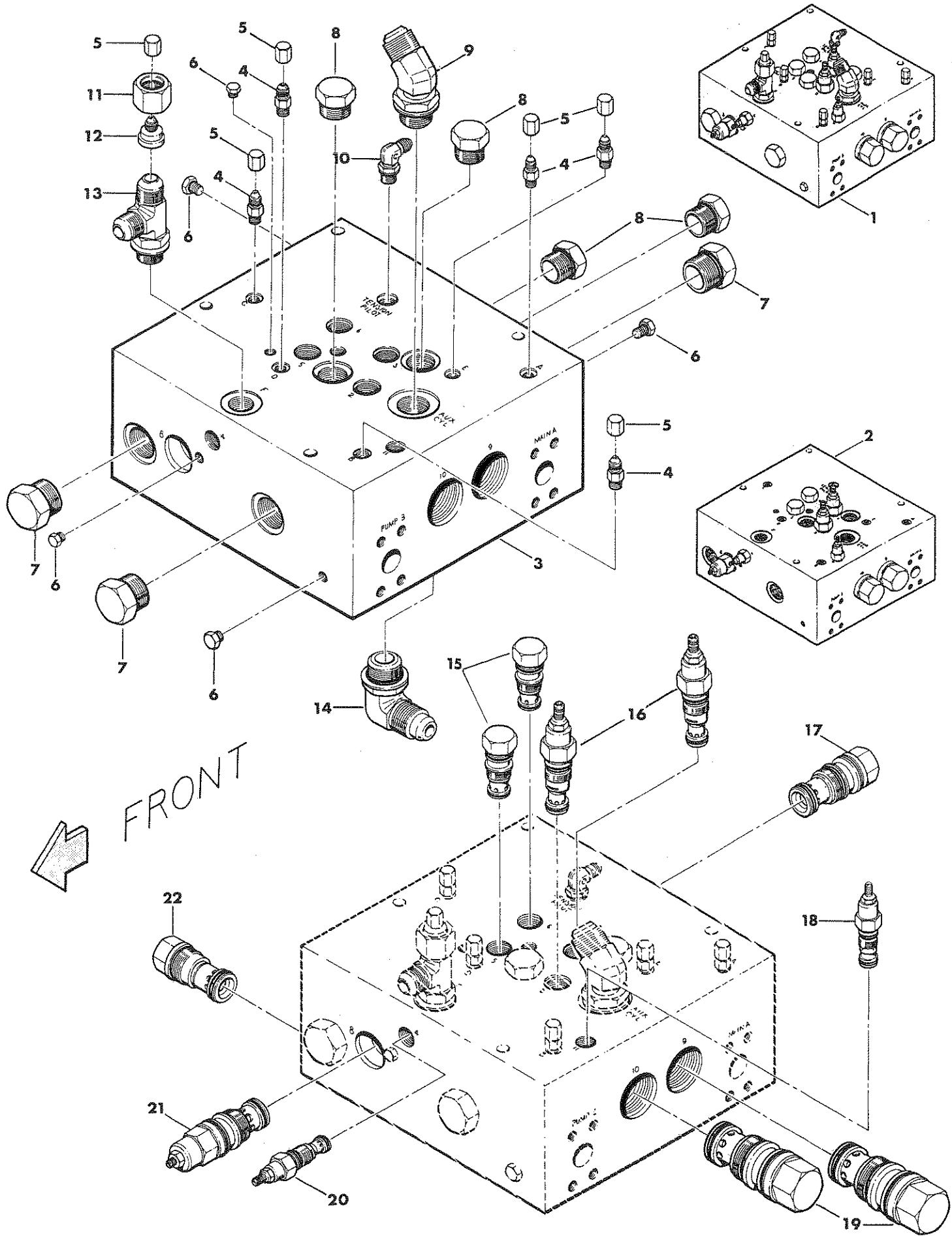
**PLUNGER CYLINDER VALVE ASSEMBLY
