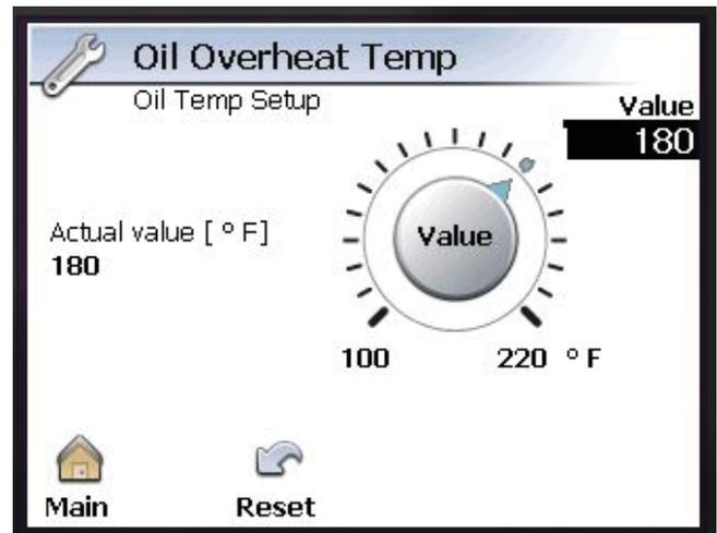
Figure 3-5-10 Oil Overheat Temp
