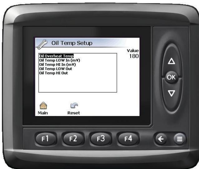
Figure 3-5-9 Oil Temp Setup
