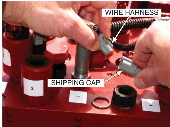
1. Remove the protective shipping cap from the male end of the wiring harness.
