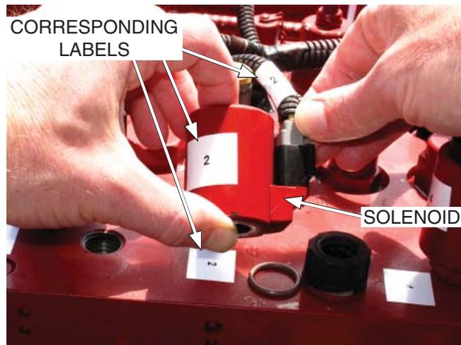
2. Push the male end of the wiring harness into the female connector on the corresponding numbered solenoid.
