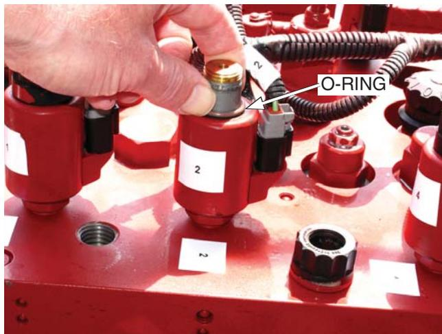
4. Carefully place the O-ring over the poppet and slide it down to the top of the solenoid.
