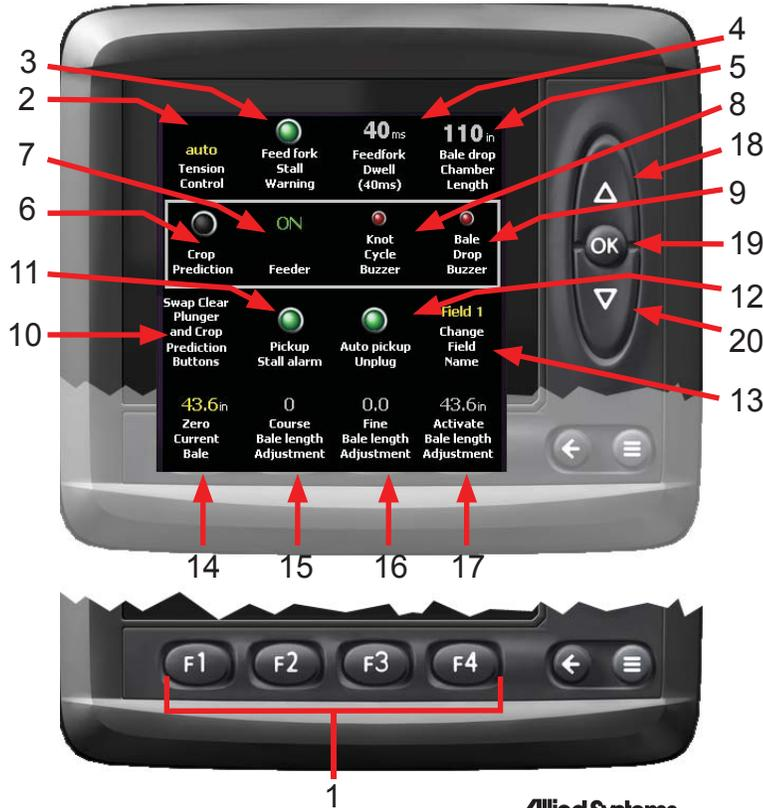
Use to scroll up and down in the menu to display all the items. The items selected for adjustment appear inside the rectangular box.
