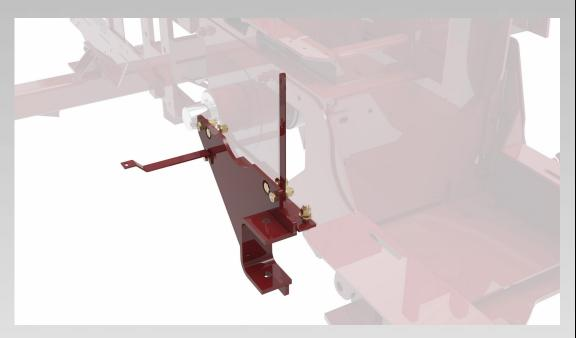
Freeman's more robust drawbar mount includes a stiffening rib for additional support. This new mount is also designed to be mounted without the use of side plate bearing housing hardware. With these improvements, the drawbar mounting bracket will last much longer under stress, which means less downtime.
