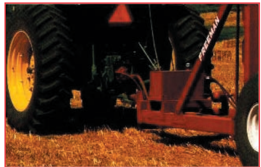
Hydraulic FF0 eliminates driveline chatter when making sharp turns.
