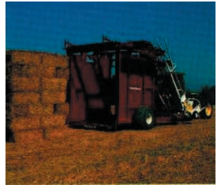
#5- Stack is unloaded, operator ready to push the reset button to automatically lower bale retainer bar and raise tilt deck into position for another load.
