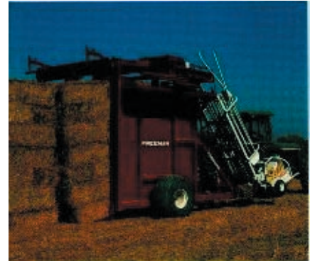
#3- Push off bar pushes stack off of tilt deck
