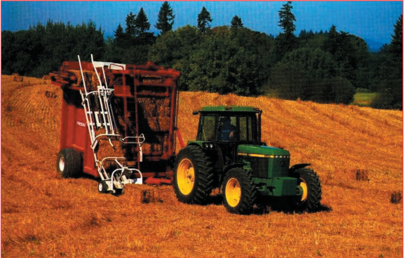
Enclosed sides on 7000 Pull Type Bale Wagon eliminates bale and stack slippage when picking up bales on hillsides.
