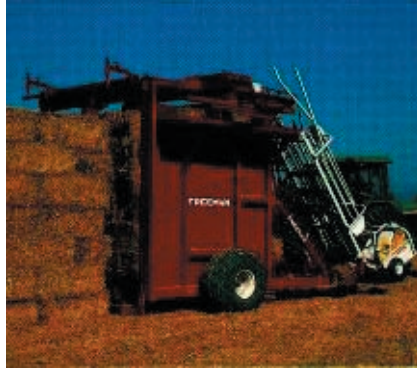
#2- Tilt deck lowered to ground and bale retainer bar raised for unloading.
