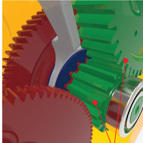
Intermediate gear and drum are free to rotate by hand.
