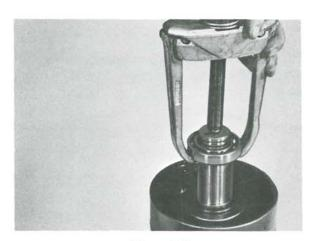
Figure 90 Remove the inner bearing.
