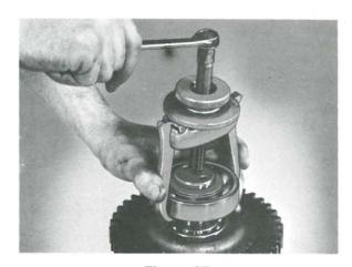
Figure 67 Remove the bearing from the shaft.
