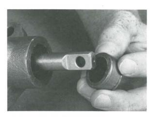
Figure 114 Apply a light coat of Permatex to the outer diameter of the valve spool oil seal. Install the lip of the seal in.
