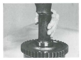
Figure 123 Install clutch gear outer bearing.
