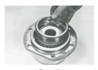
Figure 149 Install the front bearing cup in the outer race.
