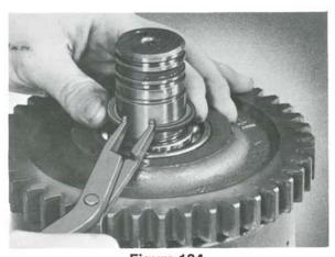
Figure 124 Install bearing retainer ring.
