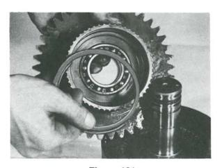
Figure 121 Install the oil baffle ring in the clutch hub gear.
