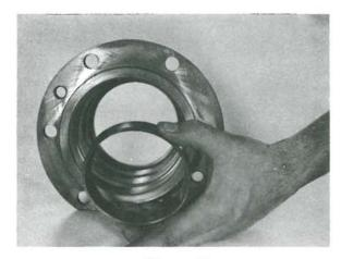
Figure 52 Remove the rear bearing cup.
