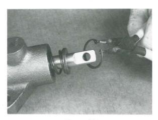
Figure 113 Compress the spring assembly and install the snap ring.
