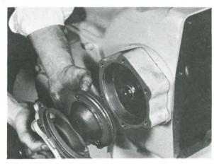
Figure 41 Remove pinion shaft piston and cover.
