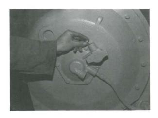
Figure 224 Install the lock button and the lock spring.
