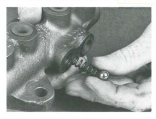
Figure 110 Insert the ball and detent spring into its location in the housing.
