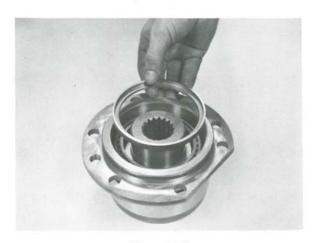
Figure 50 Remove the sprag retainer.
