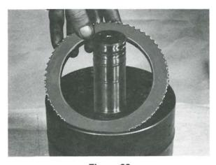
Figure 88 Remove the backing plate.
