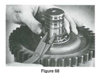
Remove the inner snap ring.
