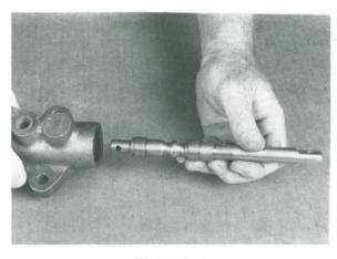
Figure 111 Insert the spool into the valve housing.
