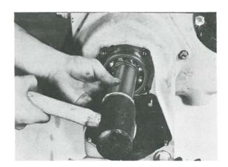
Figure 133 Install the front bearing on the clutch shaft.
