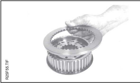
Place reaction ring onto clutch hub.
