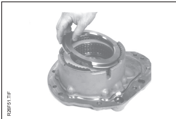
Remove the pressure plate.
