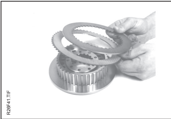
Install a friction disc onto the clutch hub and reaction ring. Follow the friction disc with a separator plate. Install the remainder of the friction discs and separator plates in the same order.
