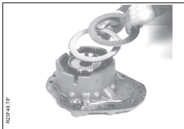
Place the ring into the housing, followed by the friction discs and separator plates.
