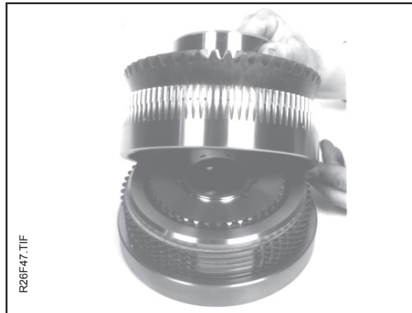
Install the clutch carrier over the clutch. Be careful not to bend or damage any of the teeth on the friction discs.
