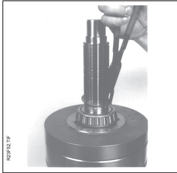
Install snap ring onto shaft.
