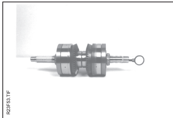
Place a lifting eye into the end of the shaft for installation into the frame.
