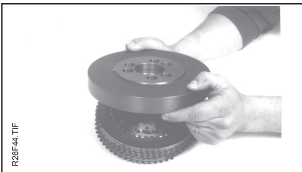
Place clutch piston housing onto the assembled clutch hub.
