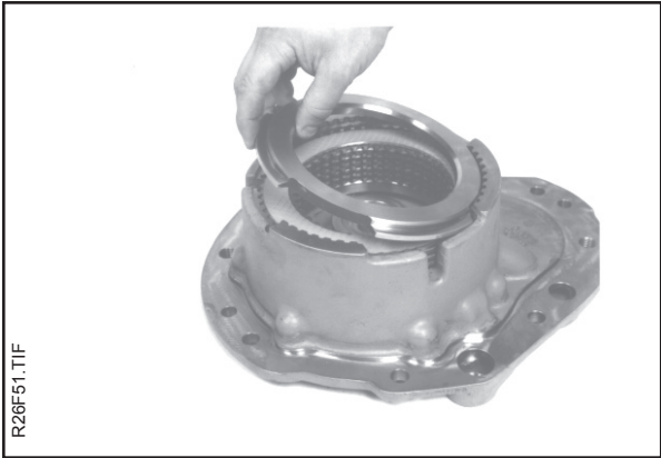
Install the flat side of the pressure plate against the last friction disc. Add the retaining ring to the brake hub to align the pressure plate.
