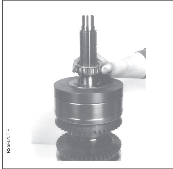
Slide bearing cone onto shaft.
