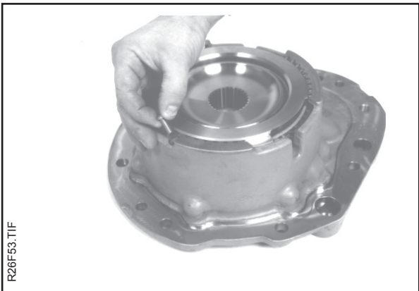
Insert and tighten the pressure plate screw in the pressure plate cut-out.
