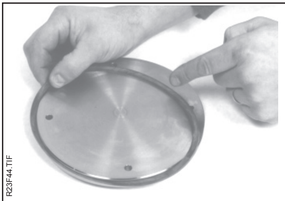
Place new seal ring on brake piston.
