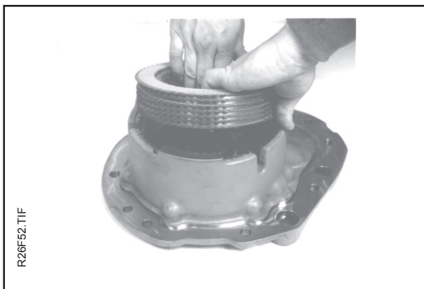
Remove the friction discs and separator plates. Inspect plate surfaces for wear and missing teeth.
