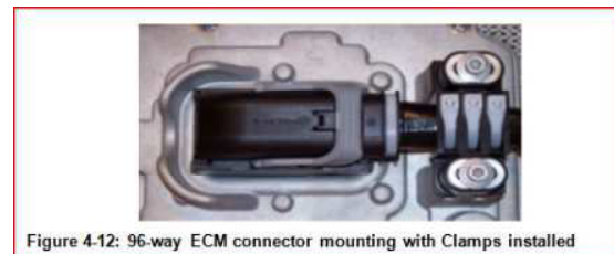
OEM CONNECTOR INSTALLED WITH CLAMP USE 3X CABLE TIES TO SECURE HARNESS TORQUE CLAMP SCREWS TO 6 IN-LBS
