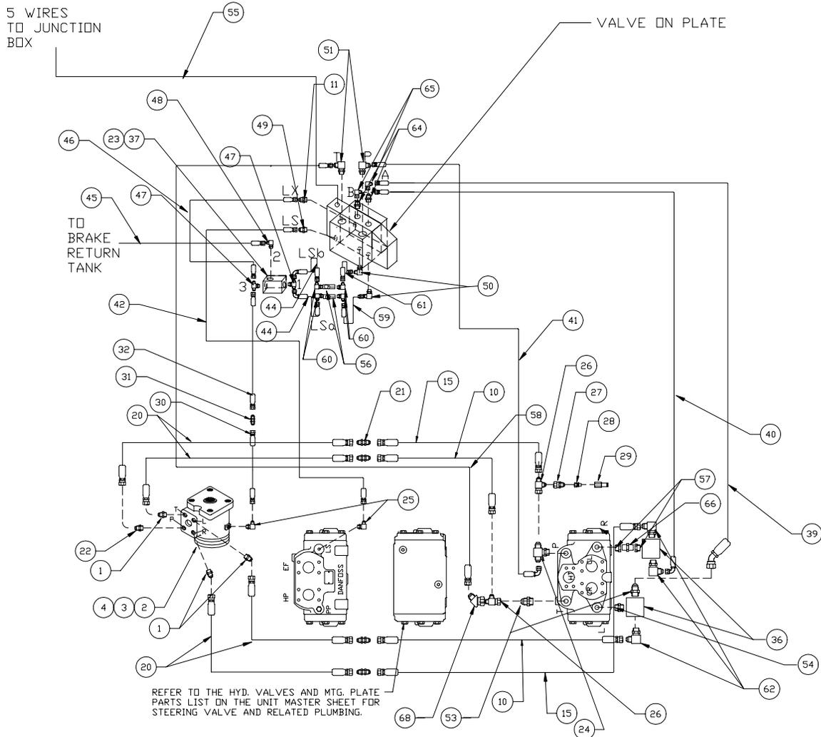
STEERING COLUMN TO VALVE PLATE
