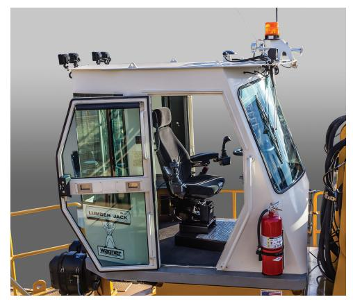
Wagner cabs include a comfortable seat and air suspension and an optional seat rotate platform for added operator comfort and safety. You can even add an optional trainer seat.
