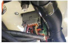
Maintenance has never been easier. Cab electrical harnesses include quick disconnect connectors.
