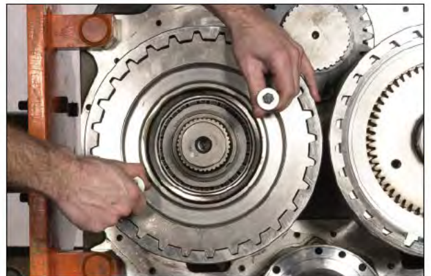
Figure 16 Install 2 bolts as shown and remove clutch piston.
