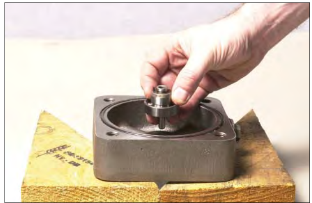
Figure 137 Remove speedo axle and bearing as an assembly.
