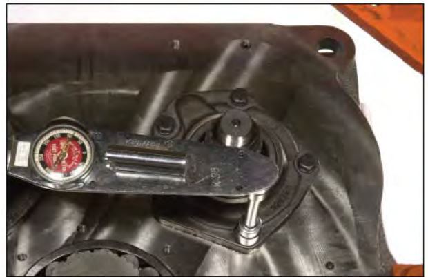
Figure 114 Install lockwashers and bolts and torque to specified torque.
