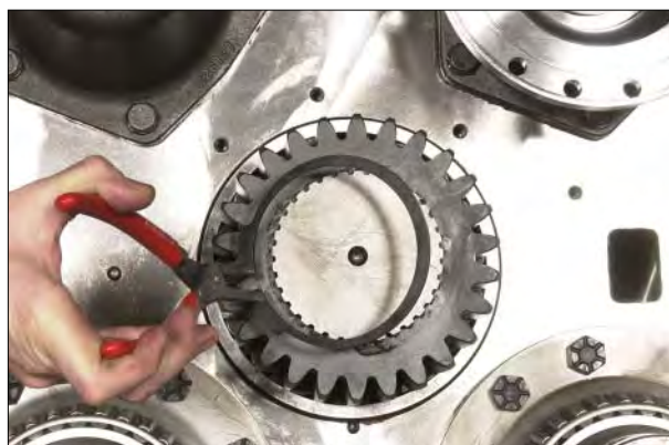
Figure 120 Install idler gear retaining snapping.
