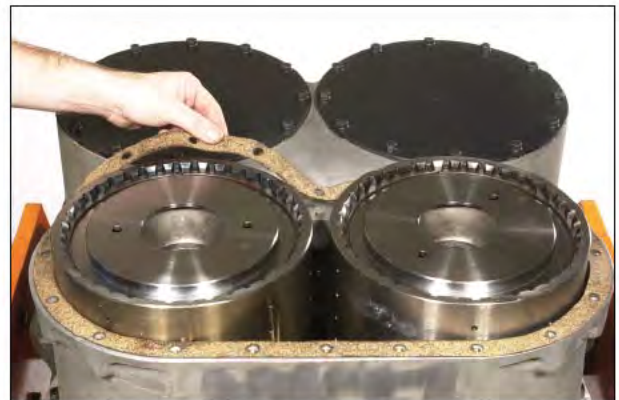
Figure 103 Install new gasket.
