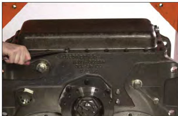
Figure 2 Remove sump pan bolts, lockwashers and oil sump pan.
