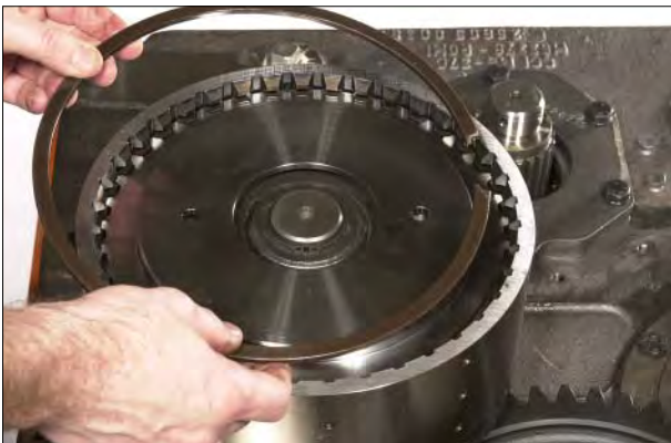
Figure 97 Install end plate retaining snapping.
