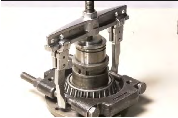
Figure 70 Remove clutch support bearing cone.
