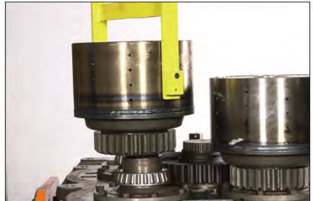
Figure 39 Hoist clutch drum from clutch support using a special tool as illustrated.
