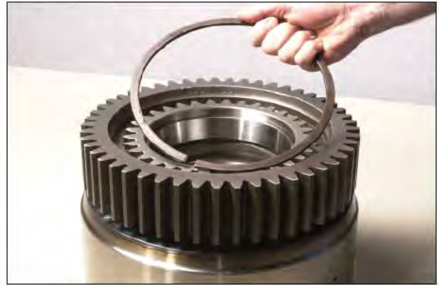
Figure 69 Instal clutch hub gear retaining snapping.
