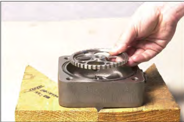
Figure 140 Install speedo drive gear.
