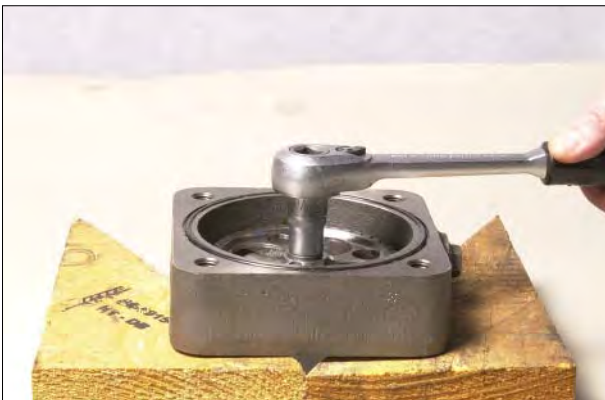
Figure 134 Remove speedo gear centre bolt
