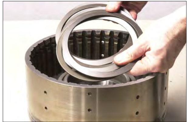
Figure 58 Remove return springs
