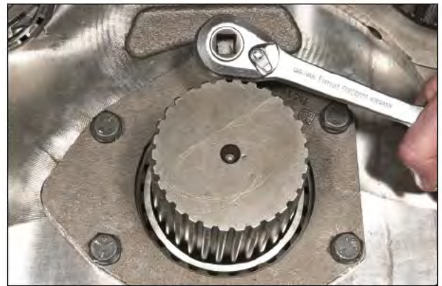
Figure 48 Remove idler shaft bearing cap.
