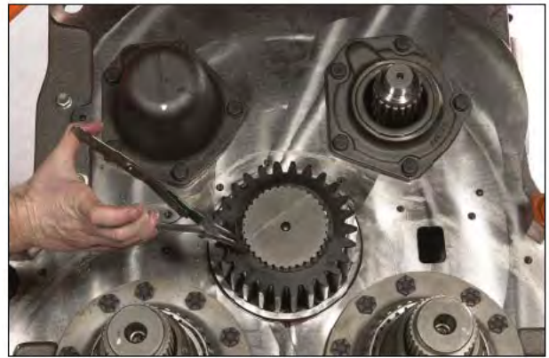
Figure 23 Remove idler gear retainnig ring.
