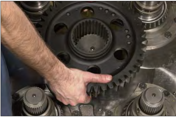
Figure 87 Install idler gear
