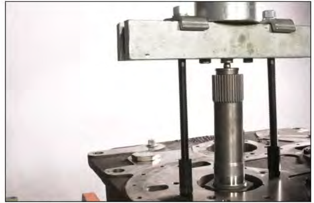
Figure 47 Using a suitable pusher tool, remove clutch shafts. Remove gears and spacers from inside of transmission case.
