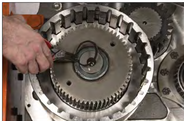
Figure 126 Install disc hub retaining snapping.
