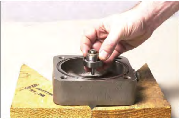
Figure 138 Install speedo drive axle and bearing.
