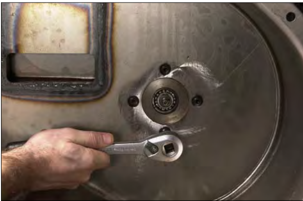
Figure 133 Speedo drive housing to case screws and sealing washers and gently tap speedo drive housing from cover.
