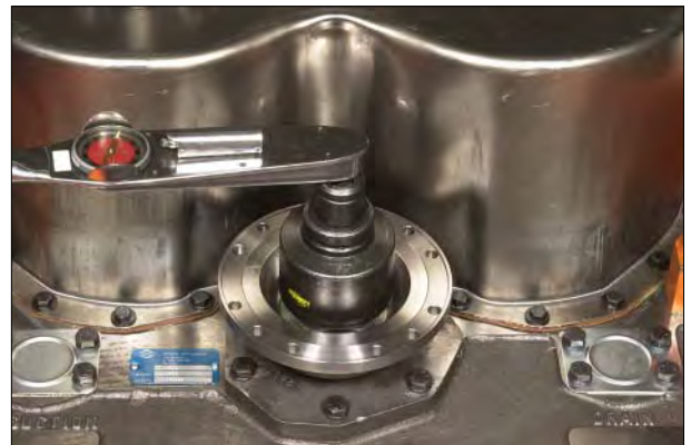
Figure 149 Torque nut to specified torque.
