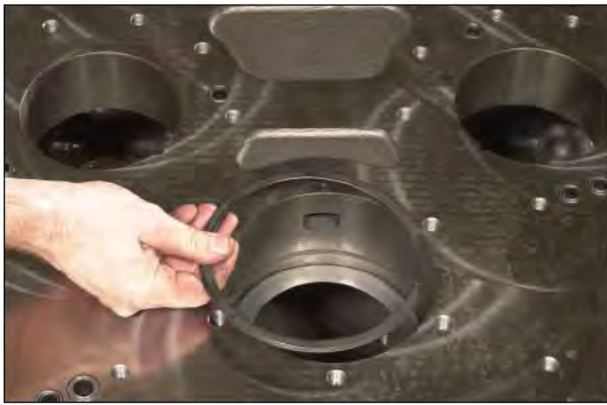
Figure 50 Remove bearing locating snap ring
