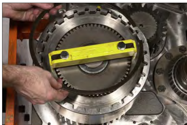
Figure 131 Use special tool to press end plate down and install end plate retaining ring.
