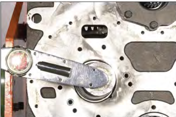
Figure 84 Torque to specified torque
