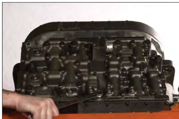
Figure 5 Remove control valve bolts and lockwashers.
