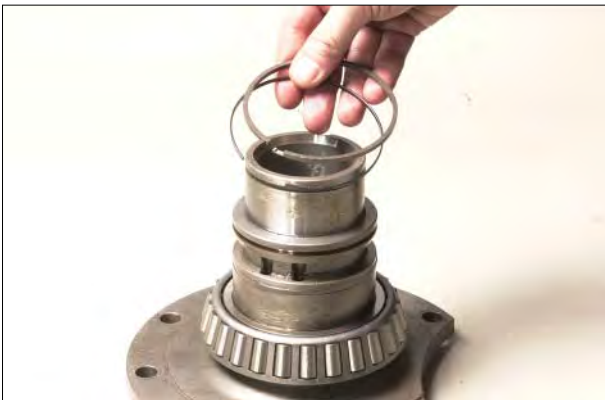
Figure 71 Remove clutch support piston rings
