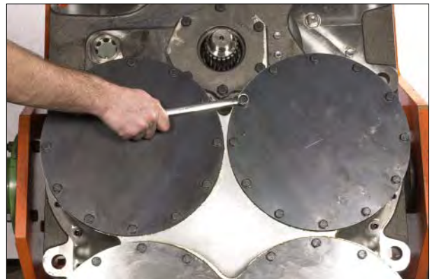
Figure 31 Remove forward, reverse, 3rd and 4th clutch cover bolts and lockwashers.
