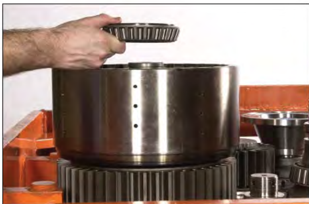
Figure 122 Install drum inner bearing cone.
