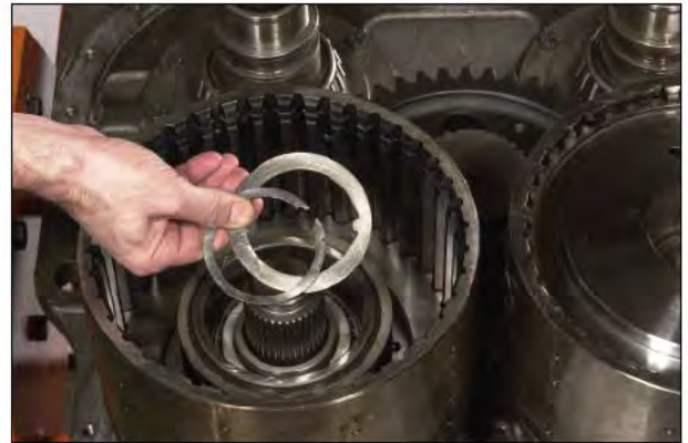
Figure 38 Remove clutch drum retainer ring and spacer.
