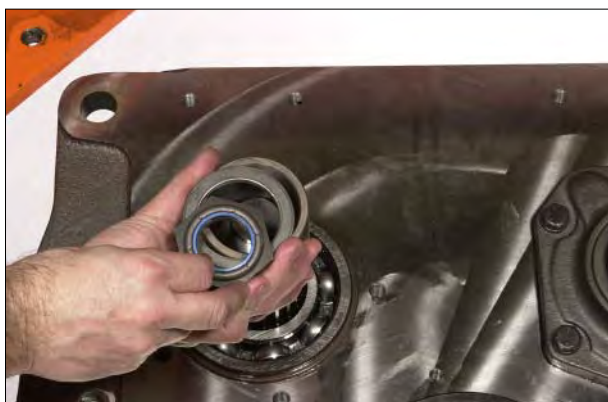
Figure 117 Install spacer, retainer and retaining nut on reverse shaft.
