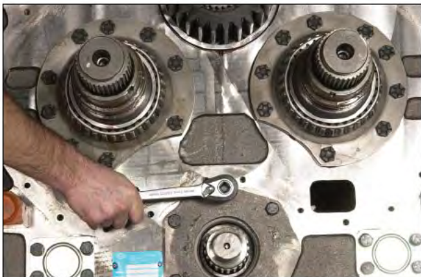
Figure 22 Remove output flange bearing cover.
