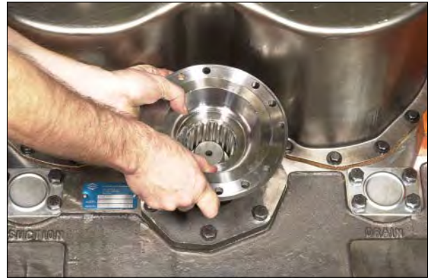
Figure 147 Install output flange.
