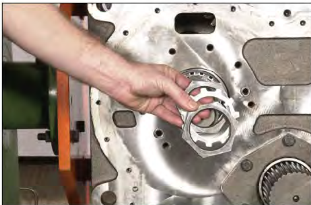
Figure 46 Straighten tongs on shaft nut locks. Lock gears with a soft bar and remove outer lock nut, nut lock and inner lock nut.
