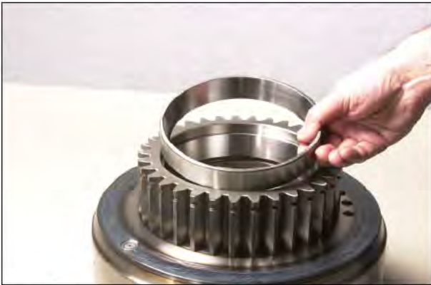
Figure 67 Install clutch outer bearing cup.
