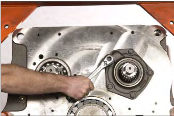
Figure 27 Remove input shaft bearing cap bolts, lockwashers and bearing cap. Remove bearing cap and oil seal.
