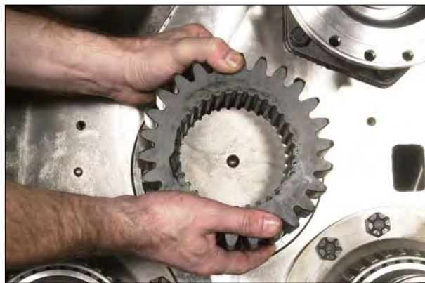
Figure 119 Install idler gear.
