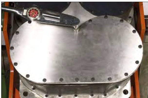
Figure 106 Place cover, lockwashers and bolts and torque to half the specified torque.
