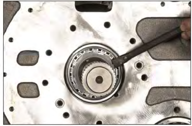
Figure 85 Secure nut loc by bending 2 lips.
