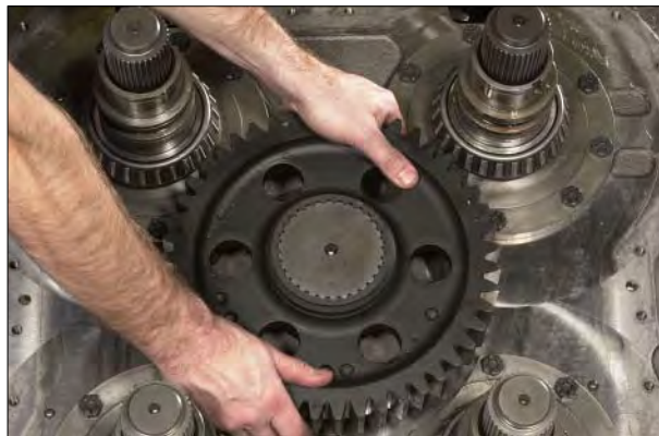
Figure 42 Remove idler gear.
