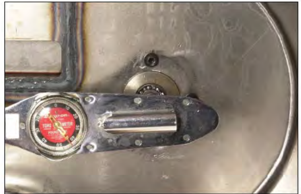
Figure 143 Install sealing washers and bolts. Torque to specified torque.
