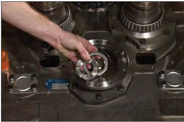
Figure 20 Remove cotter pin, output flange nut, washer and o-ring.
