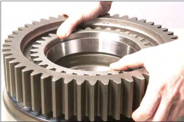
Figure 55 Remove clutch hub gear.
