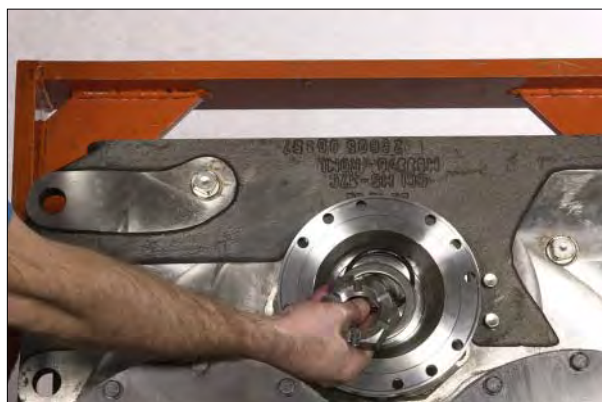
Figure 108 Install o-ring, washer and flange lock nut.
