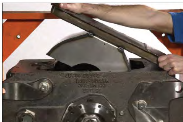
Figure 4 Remove oil sump frame and screen.
