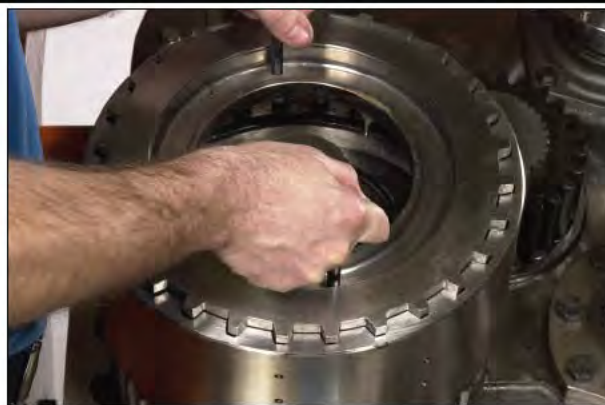
Figure 124 Install clutch piston.
