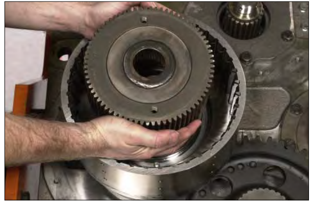
Figure 92 Install disc hub.
