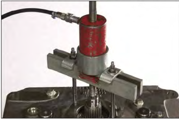
Figure 44 Press output shaft from case. Output shaft may be removed or installed from either side. Be careful! inner transmission case gears are heavy.
