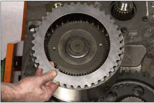
Figure 95 Install one outer clutch plate. Alternate friction and clutch plates till proper amount is reached.
