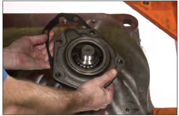
Figure 113 Install new gasket and input shaft bearing cap.
