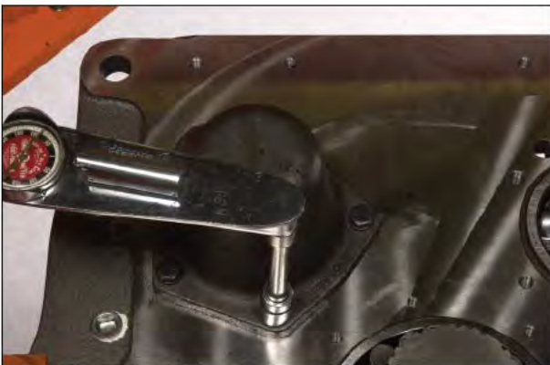
Figure 112 Place lockwashers and bolts and torque to specified torque.
