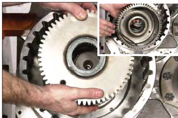
Figure 125 Install disc hub. Check that disc hub oil baffle ring is in place and intact. (See inset)
