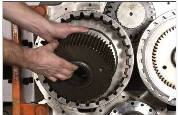
Figure 15 Remove disc hub. Remove inner and outer clutch discs.
