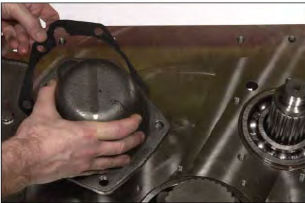
Figure 111 Install reverse shaft bearing cap gasket and bearing cap.
