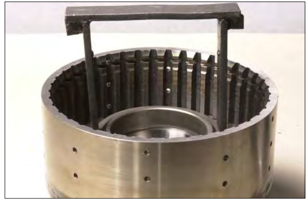
Figure 63 Install spring retaining snapping.
