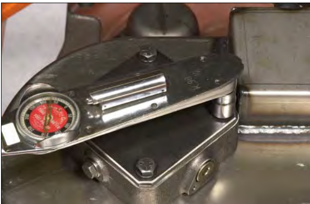
Figure 146 Install gasket and speed drive cover. Place bolts and torque to specified torque.
