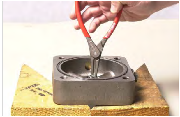
Figure 135 Remove speedo bearing retaining snapring.
