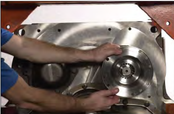
Figure 8 Remove input flange.
