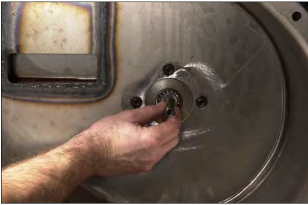
Figure 132 Remove speedo drive spring.
