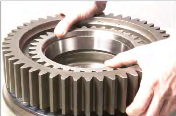
Figure 68 Install clutch hub gear.
