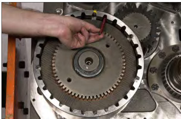
Figure 129 Install piston return springs and pins.
