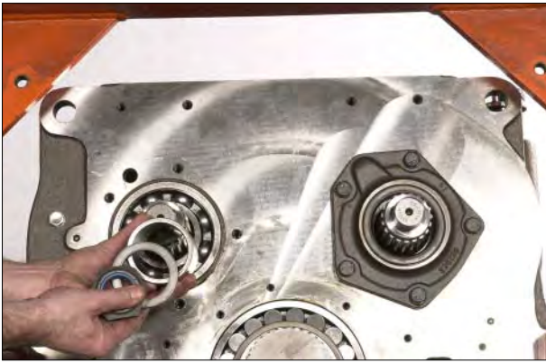
Figure 26 Remove reverse shaft nut washer and spacer.
