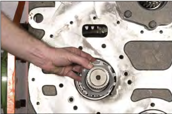
Figure 83 Install clutch drum shafts & gears. Install bearing lock nut, nut lock and lock nut.
