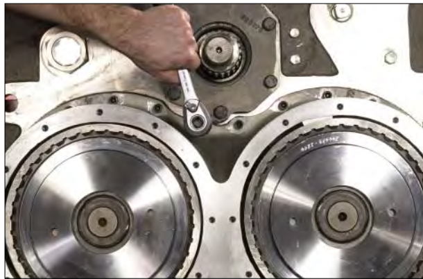
Figure 33 Remove cover base bolts, lockwashers and hoist cover base from transmission case.
