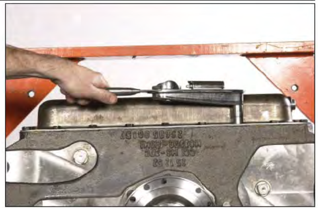
Figure 153 Install screws and lockwashers and torque to specified torque.
