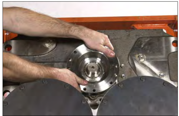
Figure 30 Remove output flange.
