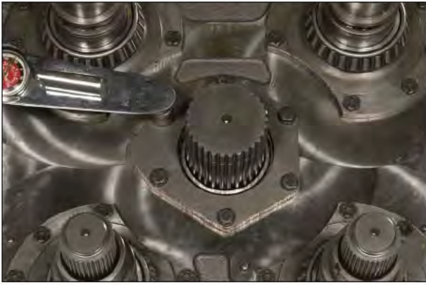
Figure 82 Install bearing cap and shims and torque bolts to specified torque. See installation procedure for shim procedure.
