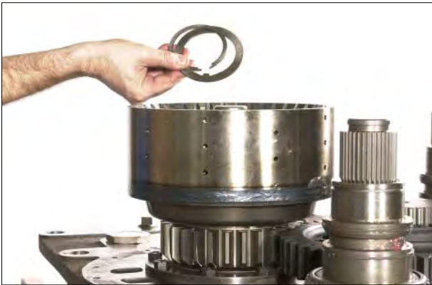
Figure 91 Install keyed washer and washer retaining snapping.
