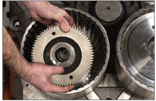
Figure 37 Remove clutch disc hub.
