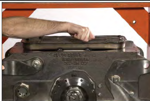
Figure 3 Remove oil screen bolts and lockwashers.
