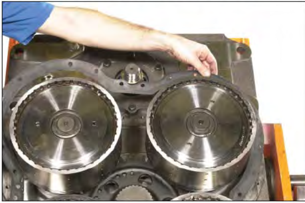
Figure 98 Install new gasket.
