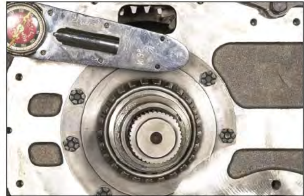
Figure 86 Install clutch support, clutch support lockwashers and screws and torque to specified torque.
