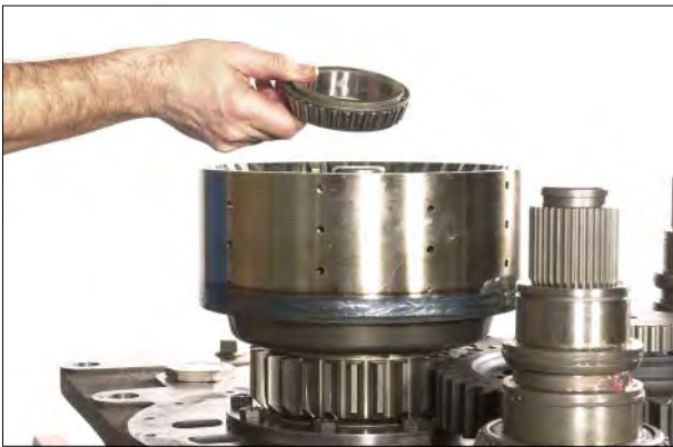
Figure 90 Install tapered roller bearing.
