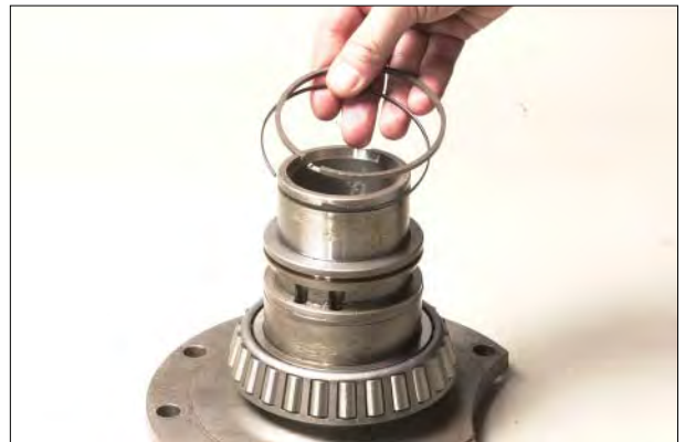
Figure 73 Install clutch support piston rings.
