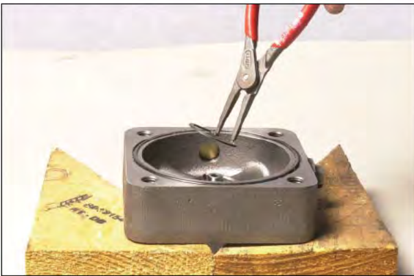
Figure 139 Install bearing locating snapping.
