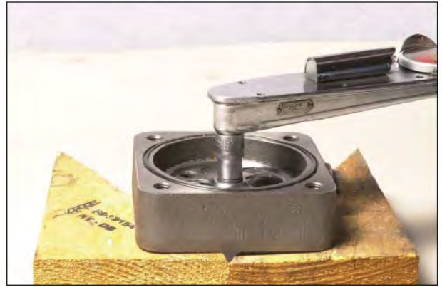
Figure 141 Install bolt and torque to specified torque.
