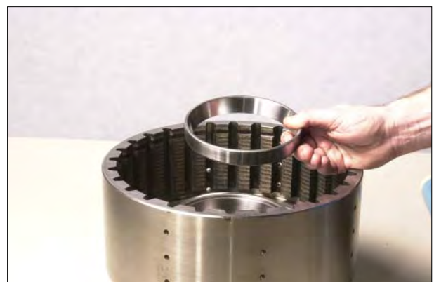
Figure 65 Install clutch inner bearing cup.
