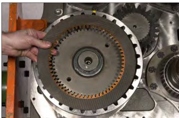
Figure 128 Install friction disc. Alternate outer disc and friction disc until proper amount is installed.
