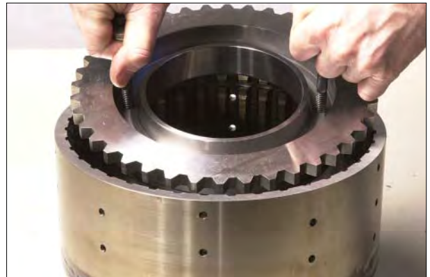
Figure 59 Use 2 bolts to remove clutch piston.
