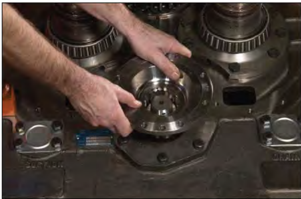
Figure 21 Remove output flange.
