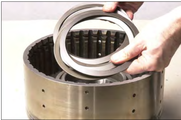
Figure 61 Install return springs. See figure 62
