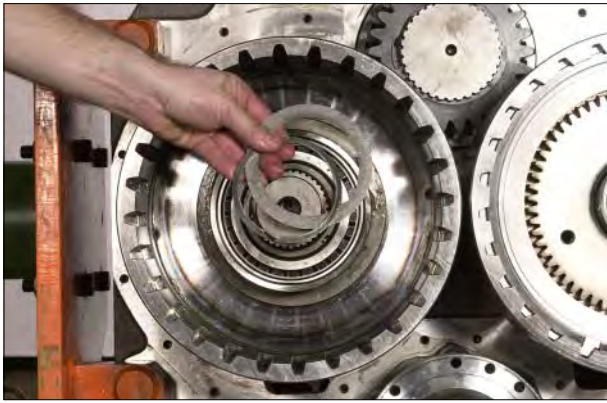
Figure 17 Remove clutch drum retaining ring and retainer spacer.
