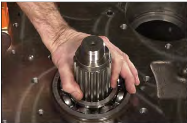
Figure 52 Remove input shaft and bearing as an assembly
