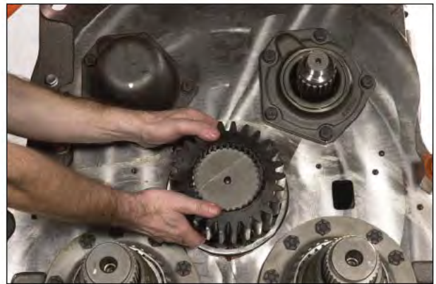
Figure 24 Remove idler gear.
