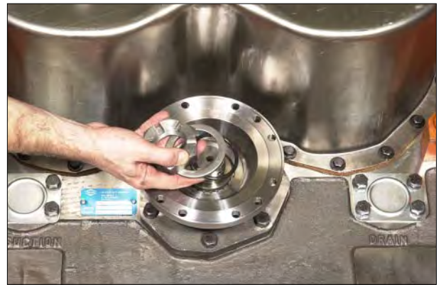
Figure 148 Install Flange o-ring, washer and lock nut.
