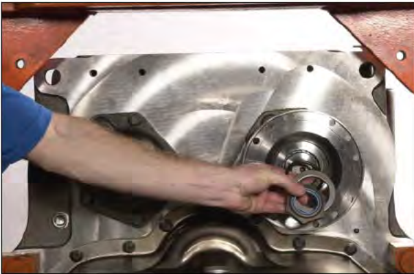
Figure 7 Remove input flange nut, washer and O-ring.
