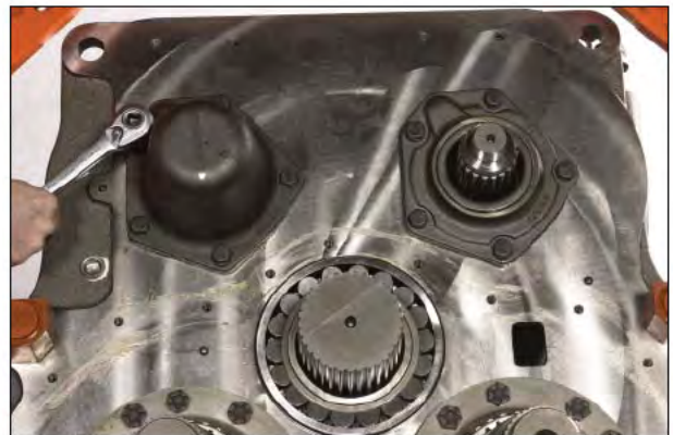
Figure 25 Remove reverse shaft bearing cap.
