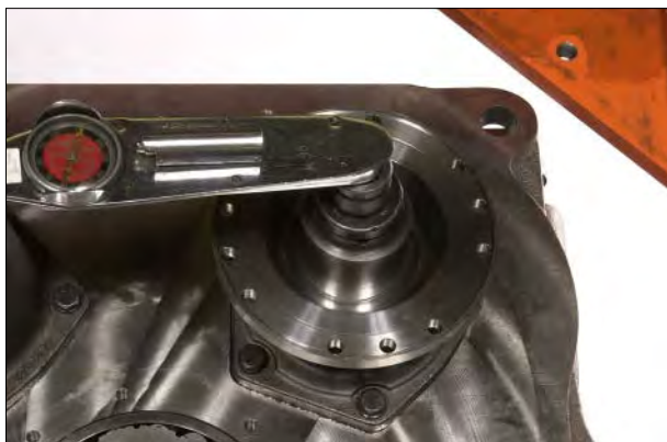
Figure 116 Install o-ring, washer and nut on input shaft and torque to specified torque.
