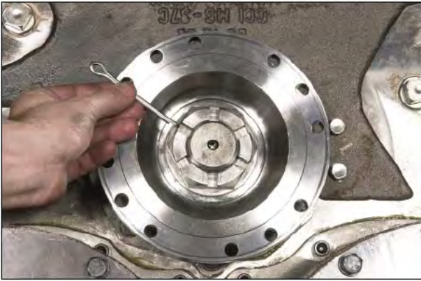
Figure 110 Install cotter pin and bend lips to secure.
