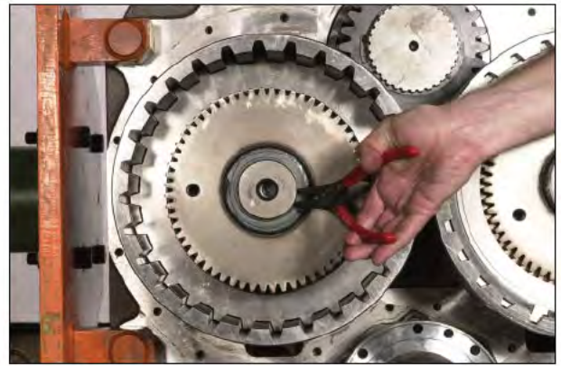
Figure 14 Remove clutch disc hub retaining ring.
