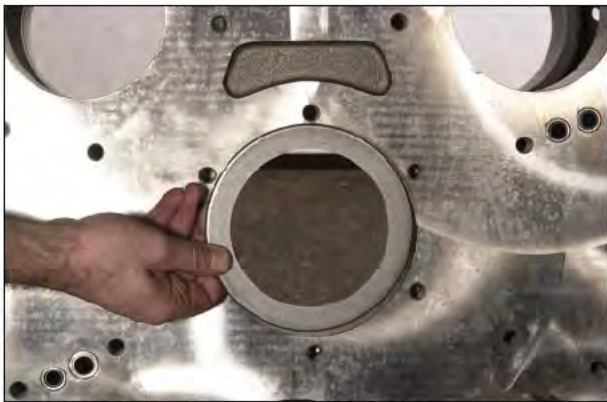
Figure 51 Remove oil shield.
