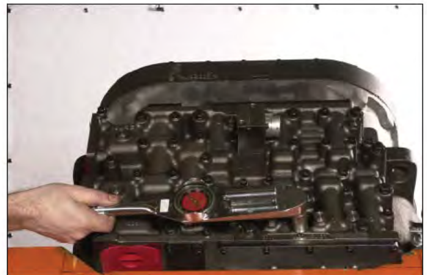
Figure 155 Install screws and torque to specified torque.
