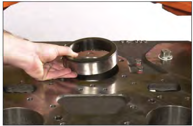
Figure 53 From other side remove bearing cup
