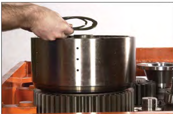
Figure 123 Install bearing washer and bearing snap ring.
