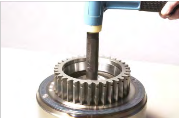
Figure 56 Remove piston ring outer race and outer support bearing cup.
