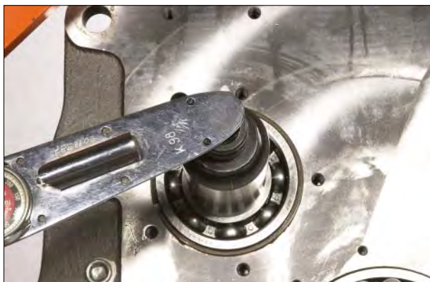
Figure 118 Torque to specified torque
