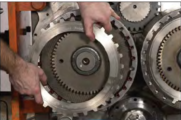
Figure 13 Remove end plate. Remove springs and pins.
