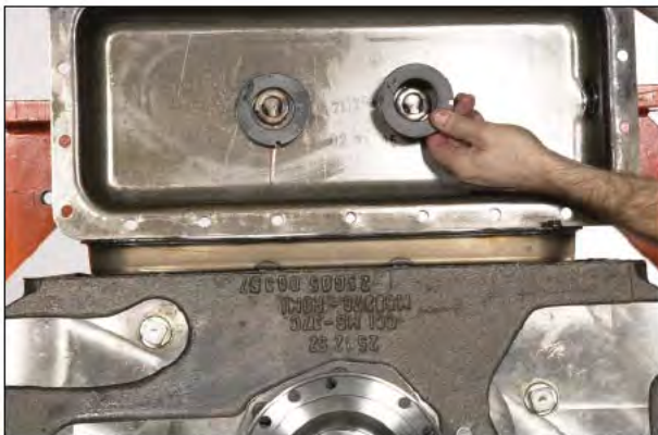
Figure 152 Clean and replace magnets in oil sump.
