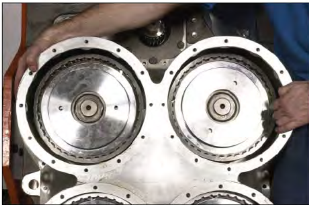
Figure 99 Use 2 aligning studs and install clutch drum cover.
