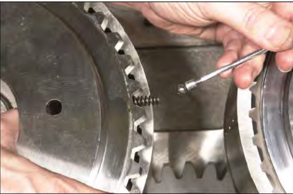
Figure 35 Locating ball and spring on either side of the end plate.
