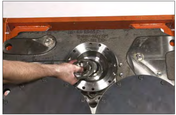
Figure 29 On other side of transmission, remove output flange nut, washer and o-ring.
