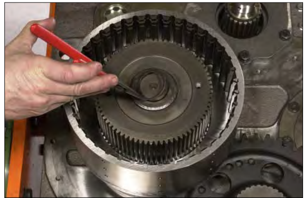
Figure 93 Install disc hub retaining ring.
