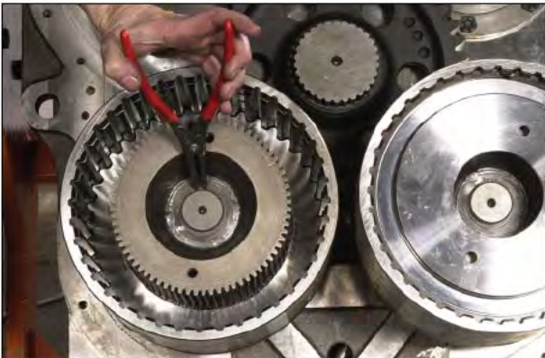
Figure 36 Remove clutch disc hub retaining snap ring.
