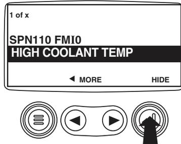
5. The display will return to the single or four parameter display, but the display will contain the "Active Fault" warning icon. Touching the "Enter Button" will redisplay the hidden fault.
