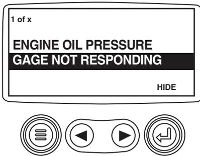
3. To acknowledge and “Hide” the fault and return to the single or four parameter display, touch the “Enter Button”.
