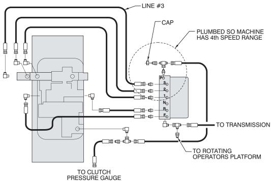
4-Speed Transmission (Optional 4th Gear Lock-Out)
