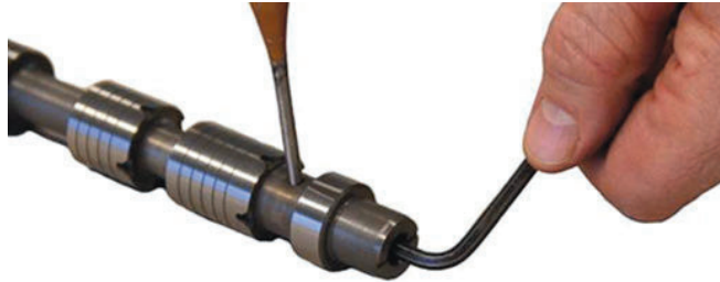
Dismantled directional spool (25) and orifice (26)
