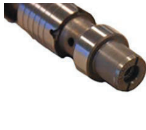
Dismantled directional spool (25) and orifice (26)
