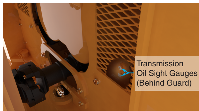
Figure 5 Transmission Oil Maintenance Location
