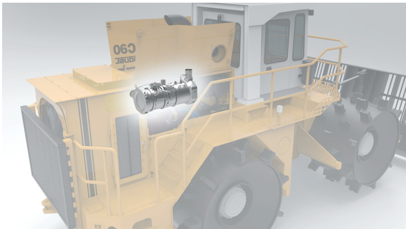
Figure 28 Diesel Particulate Filter Location
