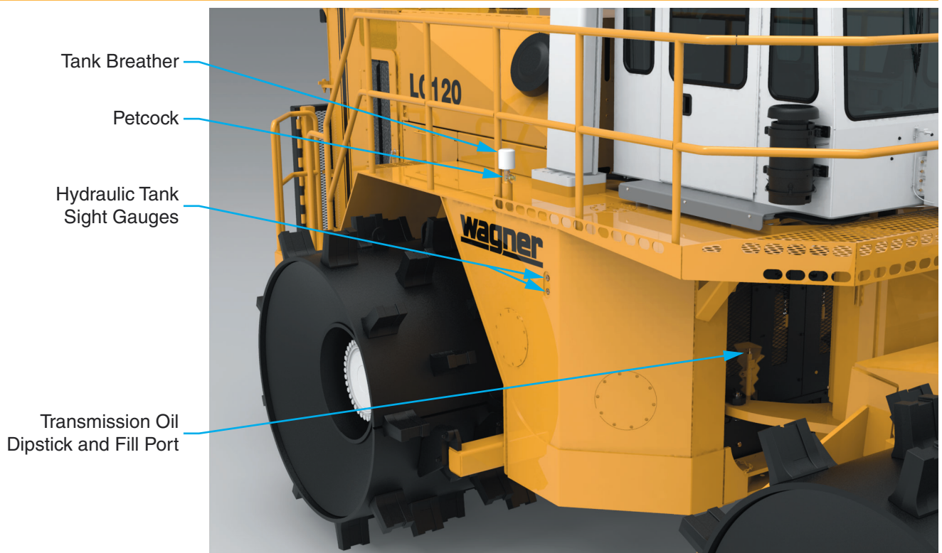
Figure 5 Hydraulic Oil and Transmission Oil Maintenance Locations
