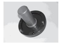
Wrench for wheel bearing adjustment nut
