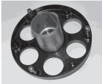
Wrench for wheel bearing adjustment nut
