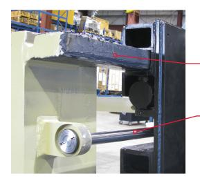
Rectangular arm slide carriers for greater load bearing surface
