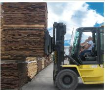
A 21,000 lb truck operating in tight aisle conditions with a heavy hardwood lumber payload.
