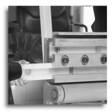
Pick a side. Insert the opposite side new outer strip into the channel by hand or by tapping with a rubber or leather mallet. **5** Next, tap in the new, long center wear strip. Continue to drive both new wear strips into the channel until they push out and replace the old, long center wear strip. Using the mallet, tap in the final new, outer piece and reinstall the plugs with mild (blue grade) 242 Loc-Tite®. Finally, torque the retainer plugs to 50 ft. lbs. and you're finished.
