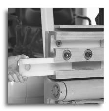
Remove the outer plugs on one side with a 3/8" ratchet. It may take a bit of effort since the plugs are torqued down to approximately 50 ft. lbs. and Loc-Tite® is installed at the factory.
