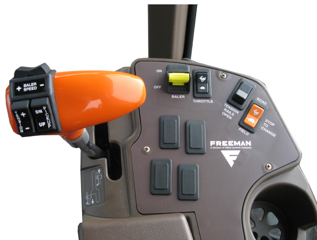
Figure 4. Armrest Control Panel
