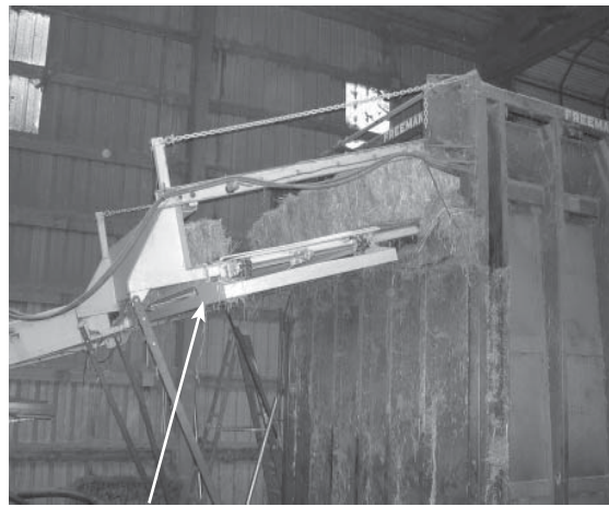
Cross feed conveyor
