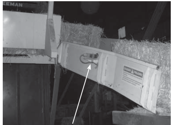
Lower bale chute photo eye Fig.11
