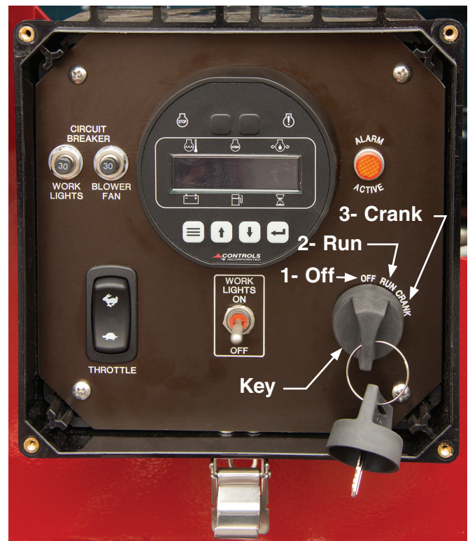
Figure 1. Engine Control Box
