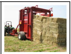
Push off bar pushes stack off of tilt deck
