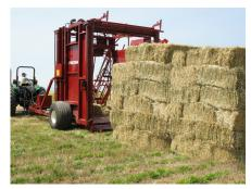
Stack is unloaded, operator ready to push the reset button to automatically lower bale retainer bar and raise tilt deck into position for another load.
