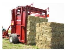
Tilt deck lowered to ground and bale retainer bar raised for unloading.
