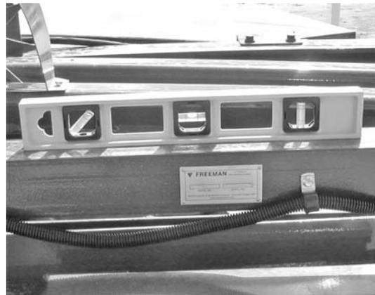
Figure 6 - Bale Chamber Level to Ground
