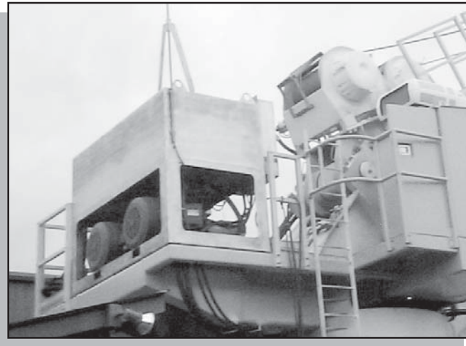
The two Lantec winches provide lots of lifting capacity in a compact unit. The two compact winches sit comfortably at the base of the 100-foot crane boom.
