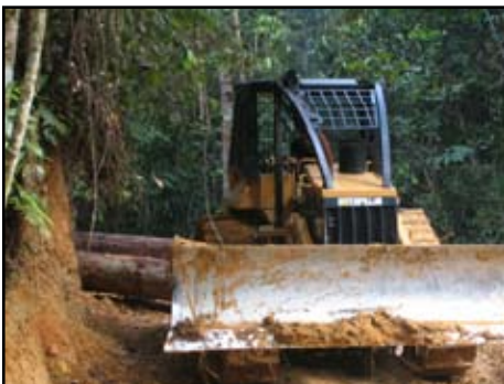
The weight-balanced W6F winch enables the Cat 527 to keep its tracks on the ground, so that it can pull two logs at a time.
