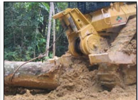
The weight-balanced W6F winch enables the Cat 527 to keep its tracks on the ground, so that it can pull two logs at a time.
