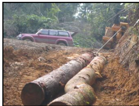
The weight-balanced W6F winch enables the Cat 527 to keep its tracks on the ground, so that it can pull two logs at a time.
