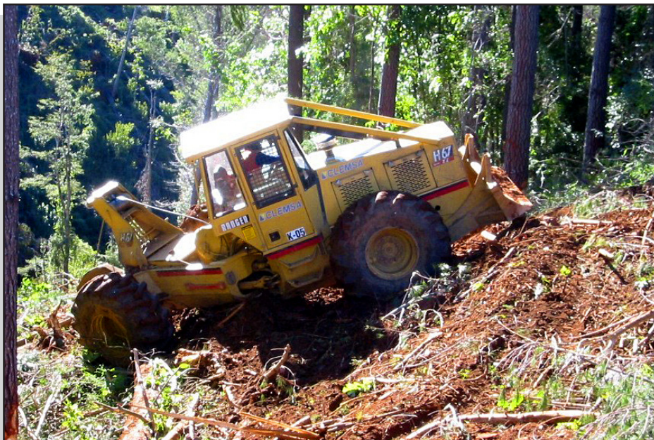
The Ranger H67, with 185 HP, clings to the mountainside near Concepcion, Chile. The stability of the skidder allows the loggers to work on steeper slopes safely.
