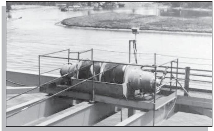
This double-ended winch provides the line pull to pull two cables on the same drum without sacrificing line speed.
