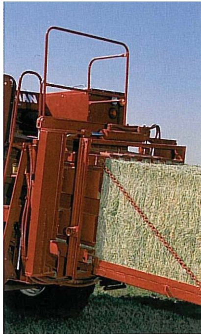
The tension control system uses four hydraulic rams to control bale density.
